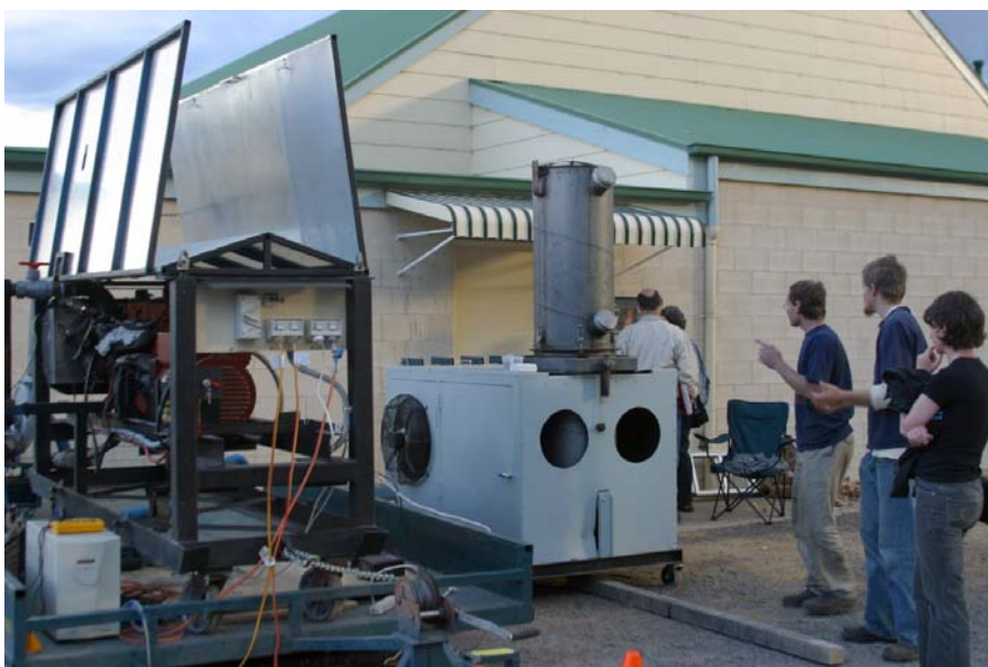
Figure 22 Proto type 15kW wood gasifier powering sustainability forum in Castlemaine
